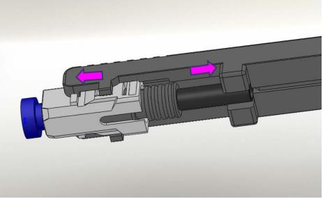
To make sure that every part is located properly, pull the slide holder to right-hand side using the tip of the thumb nail, and pull the body to left-hand side as shown in the picture above. This is the end of the procedure.
