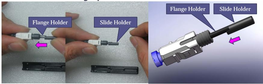
Make the flange holder wide open using the slide holder to be ready for putting the fiber, as shown in the picture above.
