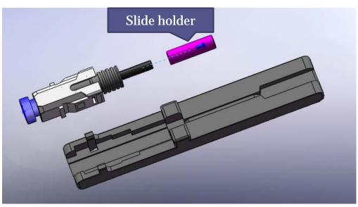
Pull out the slide holder to right-hand side, as shown in the picture above.
