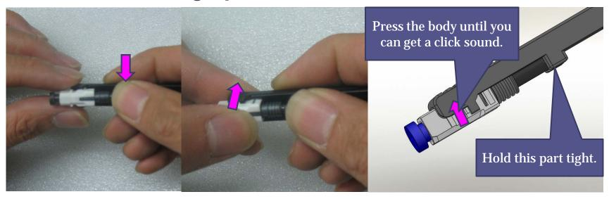
Hold tight both the end of the slide holder and the insertion guide, and press down the connector body until you can get a click sound, as shown in the picture above.
