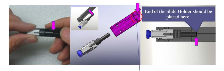
Place the end of the slide holder on the insertion guide as shown in the picture above.
